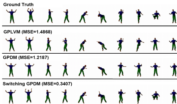
Figure 5. Exercise motion tracking results and tracking errors for three techniques.
